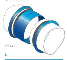
Slide the centre sleeve onto the established pipe and insert the other pipe into the sleeve to a recommended pipe gap of between 20 to 60mm. A gap is recommended in order to avoid the build up of longitudinal stresses within the two pipes as a result of thermal expansion
